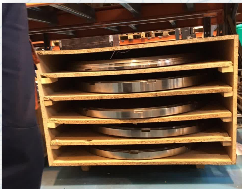
Stator ring (SGT600 Compressor)
